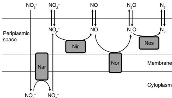
FIG. 2. Sequential reductive pathway of denitrification showing the location of enzymes relative to the cytoplasmic membrane: *Nar*, nitrate reductase; *Nir*, nitrite reductase; *Nor*, nitric oxide reductase; *Nos*, nitrous oxide reductase (modified from Ye et al. [1994]).
