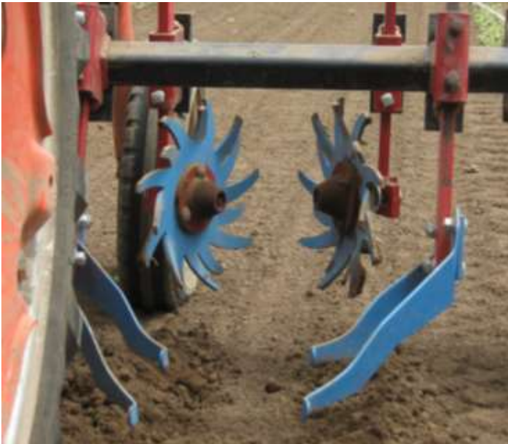
Figure 1. Spyder/torsion weeder system by Bezzerides Brothers, Inc.
