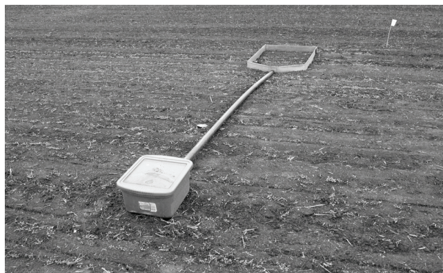
Figure 2. Runoff collector in an oat plot at the Suver site (22 Nov 03). Water and soil was collected from an area one meter square.
