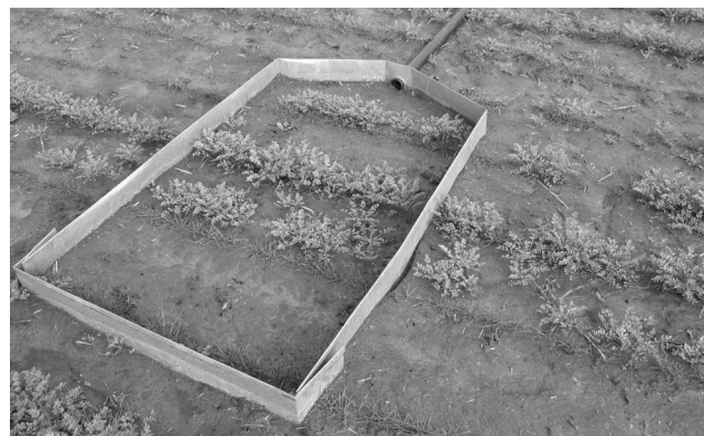
Figure 3. Runoff collector in a meadowfoam plot at Suver site (6 Feb 04). Even with a sparse stand, meadowfoam cut the runoff of soil sediment by almost half.
