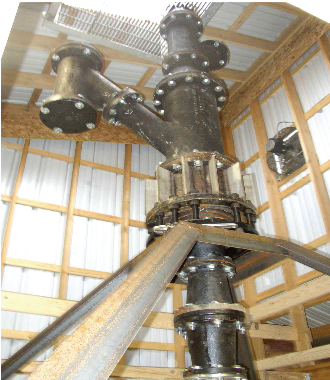
Figure 1. Taylor/WRI dual stage gasification unit used to convert straw to synthesis gas.
