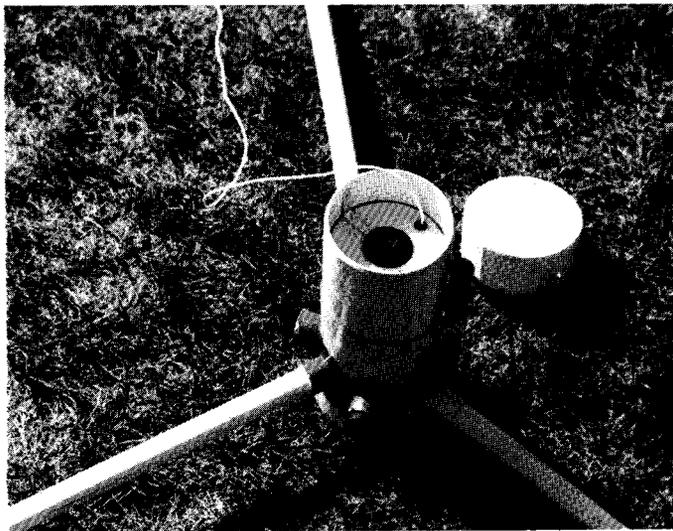
**Fig. 1.** Photograph of the assembled spider showing three legs attached to the central vertical housing. Note couplings in housing for attachment of additional legs if needed.
