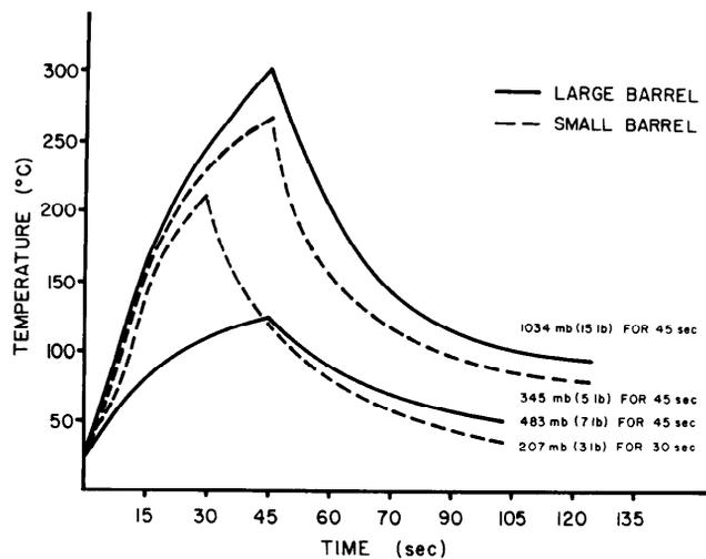
Fig. 3. Examples of time-temperature curves generated by various combinations of propane pressure and burn time for the large (107 cm) and small (58 cm) burn barrels.
