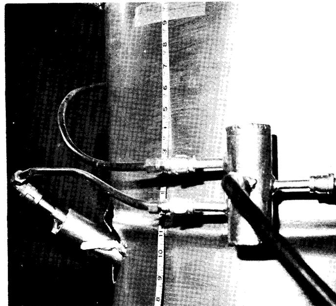
Fig. 2. Jet assembly (left) connected with copper tubing to pressure-equalization chamber (right).
