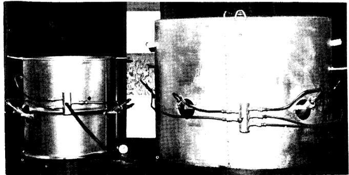
Fig. 1. Two sizes of individual plant burners. Variable pressure regulator located between the burners.
