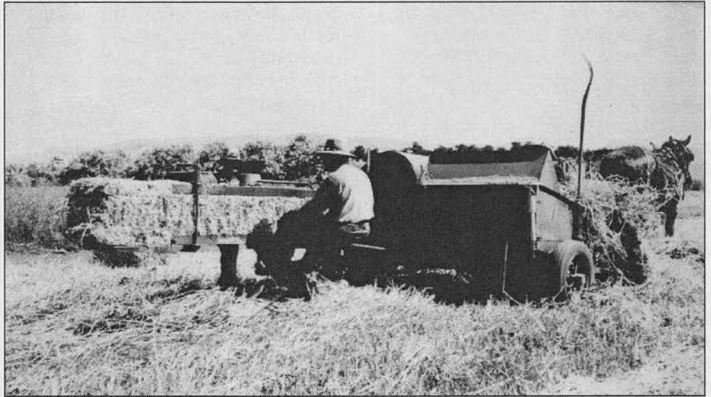
Figure 15a. Horse-drawn hay baler. During WWII, automated equipment, such as balers and elevators for stacking hay, reduced labor costs.
